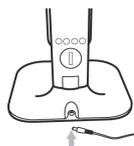
Connect the power adapter in the rear of the lamp holder
